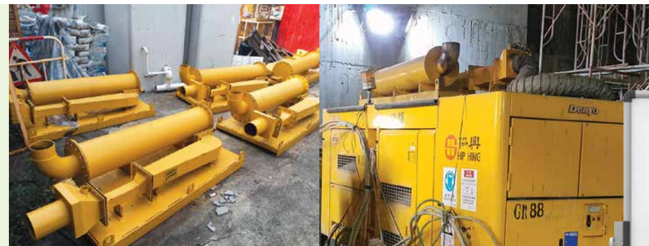
文氏旋風分離器有效去除多種有害的污染物 The Venturi Cyclone can mitigate noxious emissions effectively
