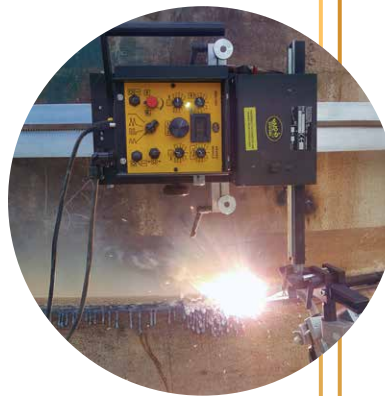
惠保開發遙控燒焊樁通系統 Remote Controlled Casing Welding Process Improvement System innovated by Vibro
