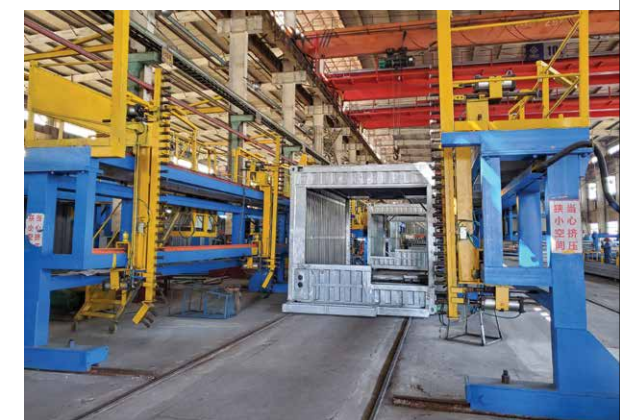
組件的製造工序轉至在較易控制的廠房環境進行 Modules are manufactured in a controlled factory environment
